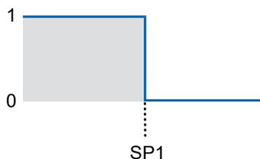
///. 6: Sensor in switching mode Point mode
